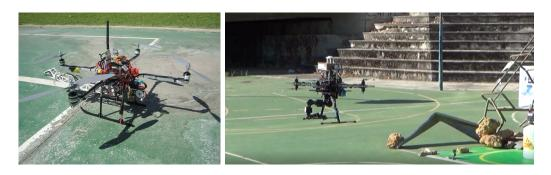
Figure 3.1: (Left)QARM1 quadrotor with three links manipulator arm developed by the University of Seville and CATEC (Seville). (Right) AMUSE octoquad aerial manipulator developed at University of Seville (AMUSE).
