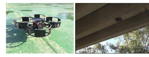
Figure 1.1: Example of a FH for bridge inspection by contact developed at the University of Seville within the AEROBI-project.
