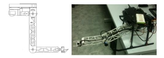
Figure 3.2: QARM1 manipulator design.
