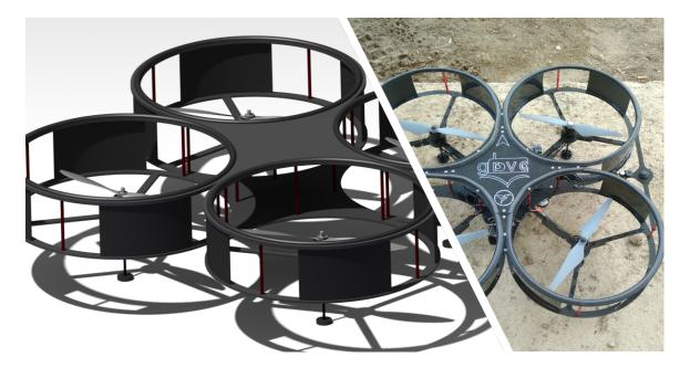
Figure 4.21: CAD of the aerial platform designed (ARBI) and the real platform developed
