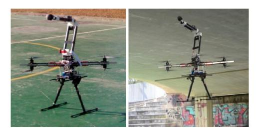
Figure 4.3: AMIS aerial manipulator for structure and bridge inspection, developed by the GRVC at University of Seville.
