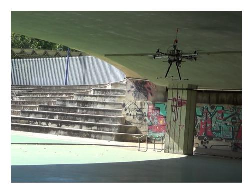
Figure 4.9: Prototype done a contact with the ceiling bridge.
