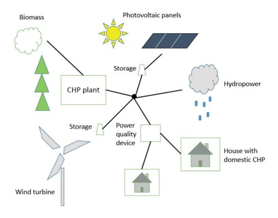
**Figure 1.** Decentralized energy production by using renewable energy (modified from Vezzoli et al. 2018). Large centralized power plants are replaced by smaller interconnected production units.
