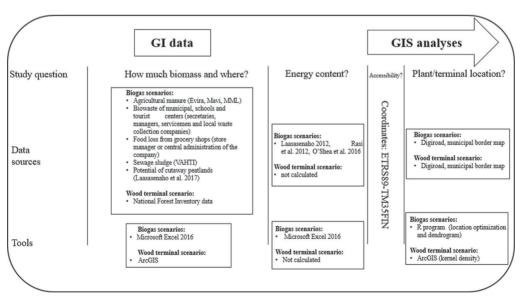
Fig. 4. GIS process for determining the optimal locations of biogas plants and wood terminals in the study area. Four GIS-related questions are answered using biomass data and different GIS tools.
