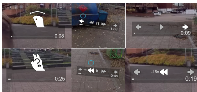
Figure 1: UI elements for gestures (left), head pointing (middle), and remote control (right).
