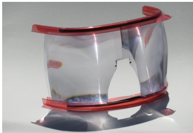
Figure 2. Super-wide-FOV curved Fresnel mask prototype
