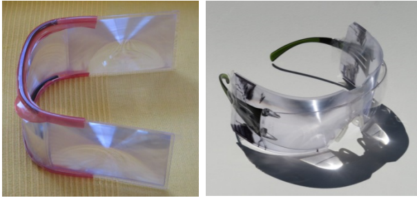
Figure 4. Left: World's widest FOV (343° diagonal). Right: Fresnel lenses curved around safety glasses (FOV: 293° diagonal)
