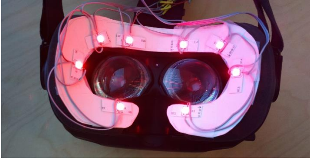
Figure 2: The LED face skin mask is beyond FOV and does not obstruct the HMD view.
