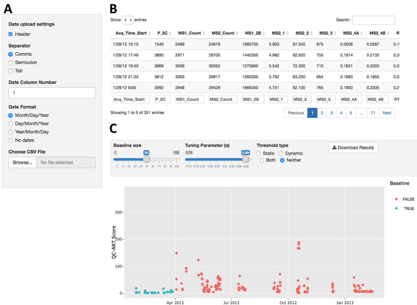
Fig. 6. QC-ART interface. A , Data upload and settings. B , Verification of the uploaded data. Once the data are uploaded they can be verified and searched. C , Results and output. The results can be visualized in the interactive graph and downloaded as a comma separated file. Tuning parameters, including baseline size, can be adjusted by experienced users to better discriminate poor-quality runs.
