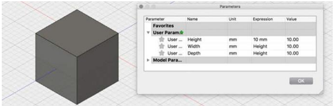
Figure 21 Cube created with parametric modeling [20].
