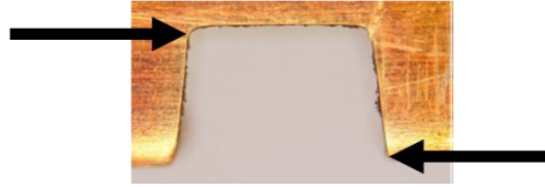
Figure 60 Residual burr in cut.
