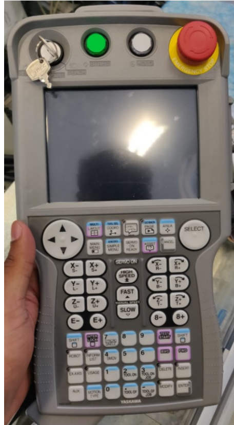
Figure 1 Teach Pendant Yaskawa Motoman robots
