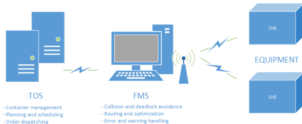
Figure 5: Container terminal's control system [42]
