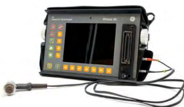
Figure 9. Ultrasonic inspection equipment (Phasor XS 16/16 Olympus).
