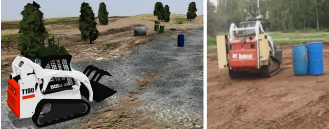
Figure 7. On the left a view from Gazebo simulation environment; on the right RobIL UGV avoids an obstacle autonomously. (Meltz and Guterman, 2019) © 2019 IEEE.
