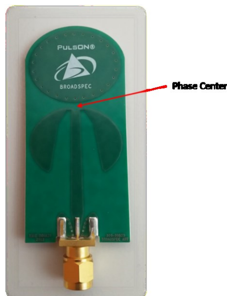
Figure 12. Broadspec antenna with the Phase Center indication
