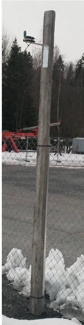
Figure 18. Installation of a reference node around the test area
