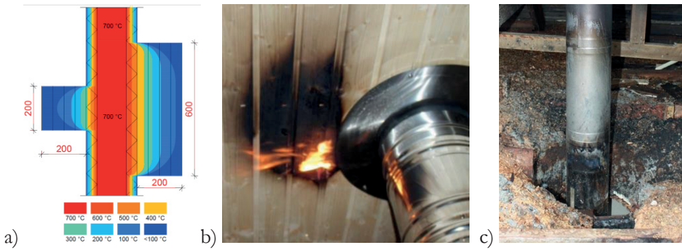
Figure 1.3 a) An example of the temperatures at the penetration of the chimney. The chimney locates in the middle of the figure. On the left side of the chimney is an insulation layer 200 mm thick and on the right side the insulation thickness is 600 mm. The temperatures are based on experimental measurement results. b) Ignition from the penetration of the metal chimney. c) Chimney roof penetration after fire.
