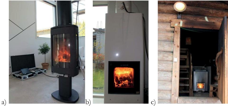
Figure 3.7 The fireplaces tested in field experiments: a) Room heater and site measurement equipment, b) Slow heat release appliance, c) Exterior view of lakeside sauna and sauna stove.
