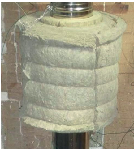
Figure 1.4 a) Test structure, b) Effect of thickness of roof insulation on the temperatures of penetrations [Inha et al. 2011]. Temperatures are measured at a distance of 100 mm from the chimney's outer surface.
