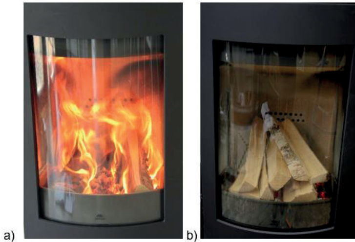
Figure 6.1 a) Normal wood batch (1.4 kg). b) A wood batch twice as large (2.8 kg).
