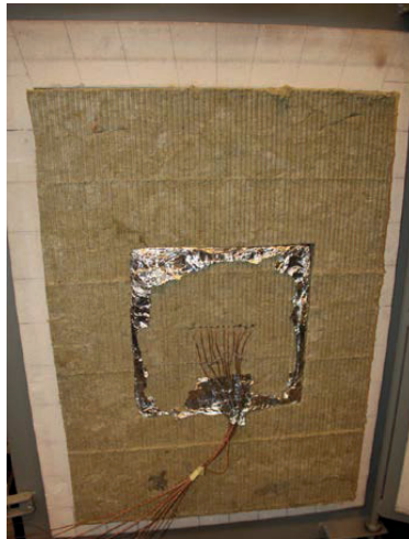
Figure 7. Test specimen installed in the wall of the furnace.
