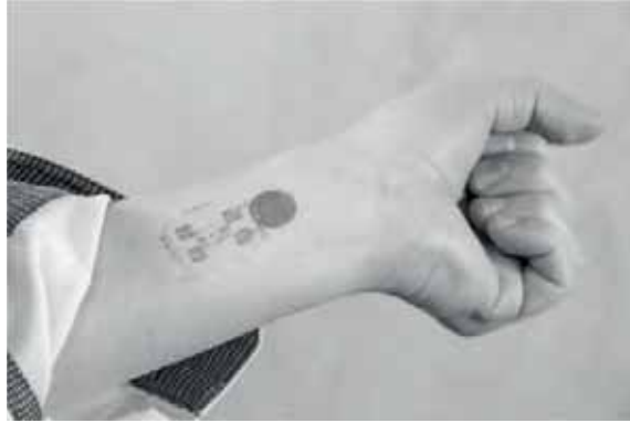
Figure 18: Proposed ultra-thin lab-on-skin setup with printed piezoelectric biosignal sensor and integrated charge amplifier.
