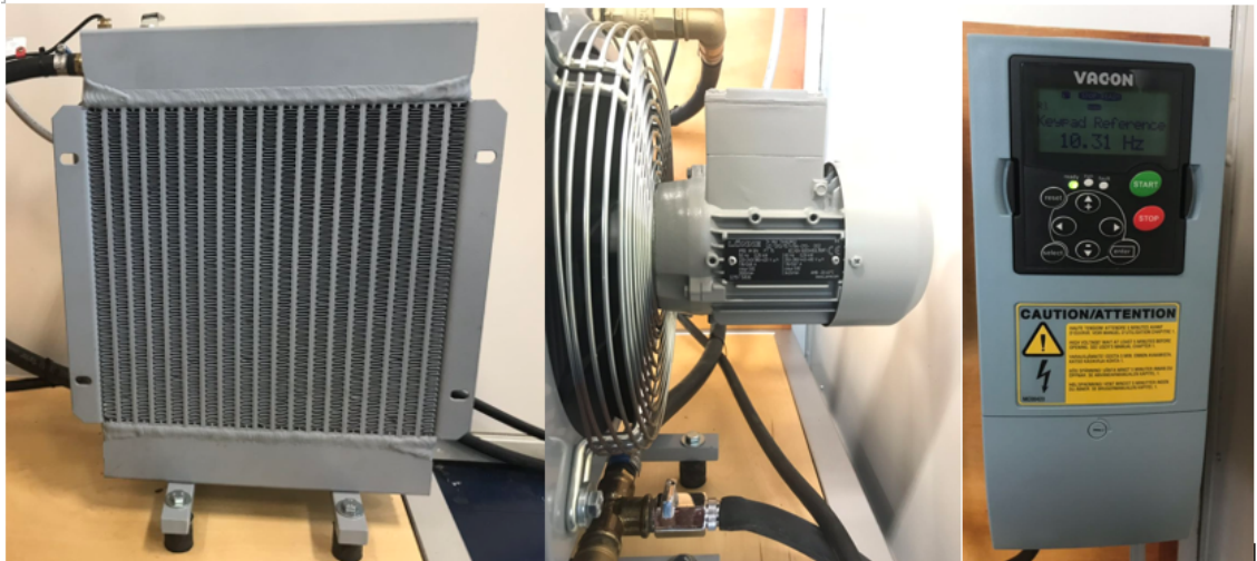
Figure 5.5. Air cooling system
