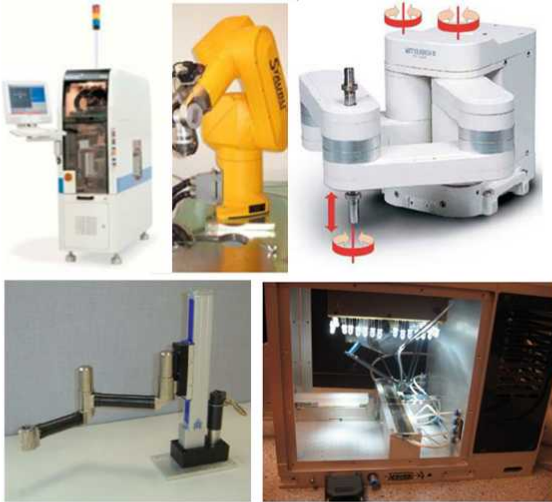
Figure 10. Machines used for power consumption measurements, from upper left corner: Hisac 500 OF, Stäubli RX60, Mitsubishi RP-1AH, Schunk desktop scara (prototype), Pocket Delta (prototype). Images are not in same scale. (images from Escribano Gimeno, 2010)
