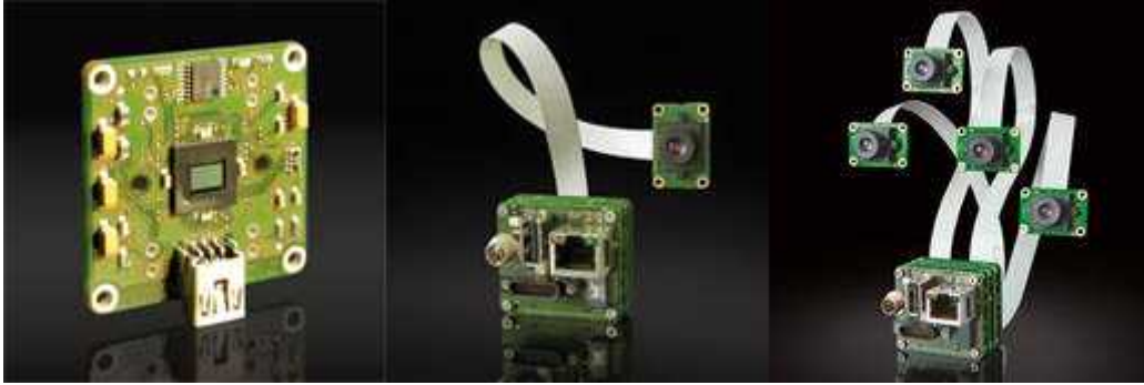
Figure 39. Board level camera (32 x 32 x 7 mm) without optics connector and camera system with one or up to four remote camera heads (remote head boards 28 x 19 mm, central unit about 42 x 38 mm). Remote camera heads use user selectable lens mounts. ( http://www.vrmagic.com/ )
