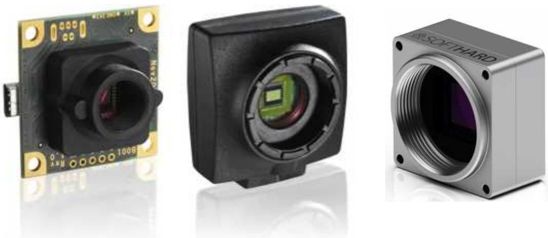
Figure 38. Board level camera (36 x 36 x 20 mm) with S-mount optics connector and enclosed camera (44 x 44 x 25 mm) with normal C/CS-mount for optics. Both have USB 2 interface. ( http://www.ids-imaging.com/ ) On right, “subminiature” camera (size 16x16x13 mm) with M12 lens mount from Ximea ( http://www.ximea.com )
