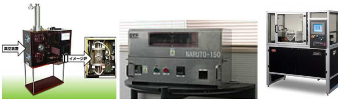
Figure 15. Ultra Compact Hot Embossing Machine (see DTF, 2011), Desktop Nickel Plating Machine (ibid.), Nanomolding machine Sesame (Medical Murray, 2011)
