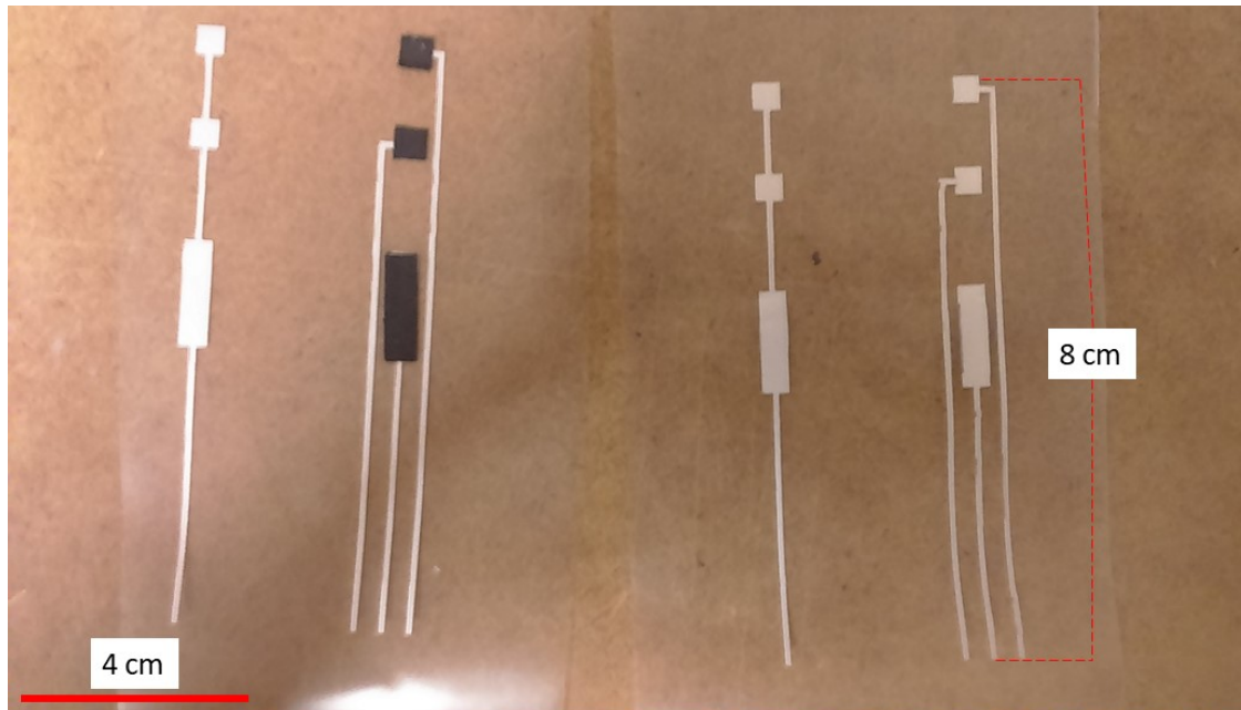
Figure 23. Captured image of the printed electrodes and the laser-patterned piezoresistive fabric
