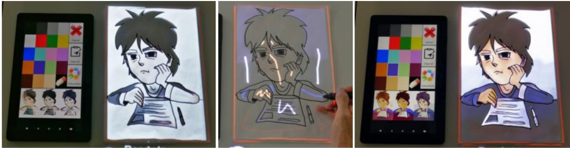
Figure 11: The user-AI collaboration process of ColorAIze. From left to right: initial colourisation; user adding local color hint; result generated by AI (Matulic, 2018)
