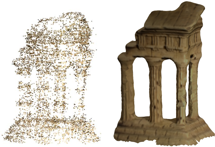
Figure 4.10. Point cloud built from the patch model and the final textured model.
