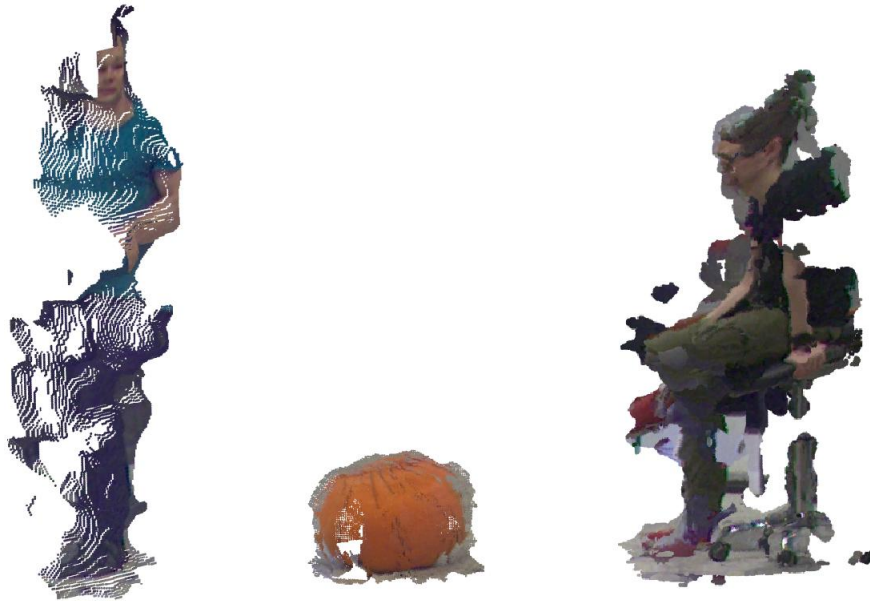
Figure 4.5. Examples of the rough 3D object models segmented from the global point cloud.
