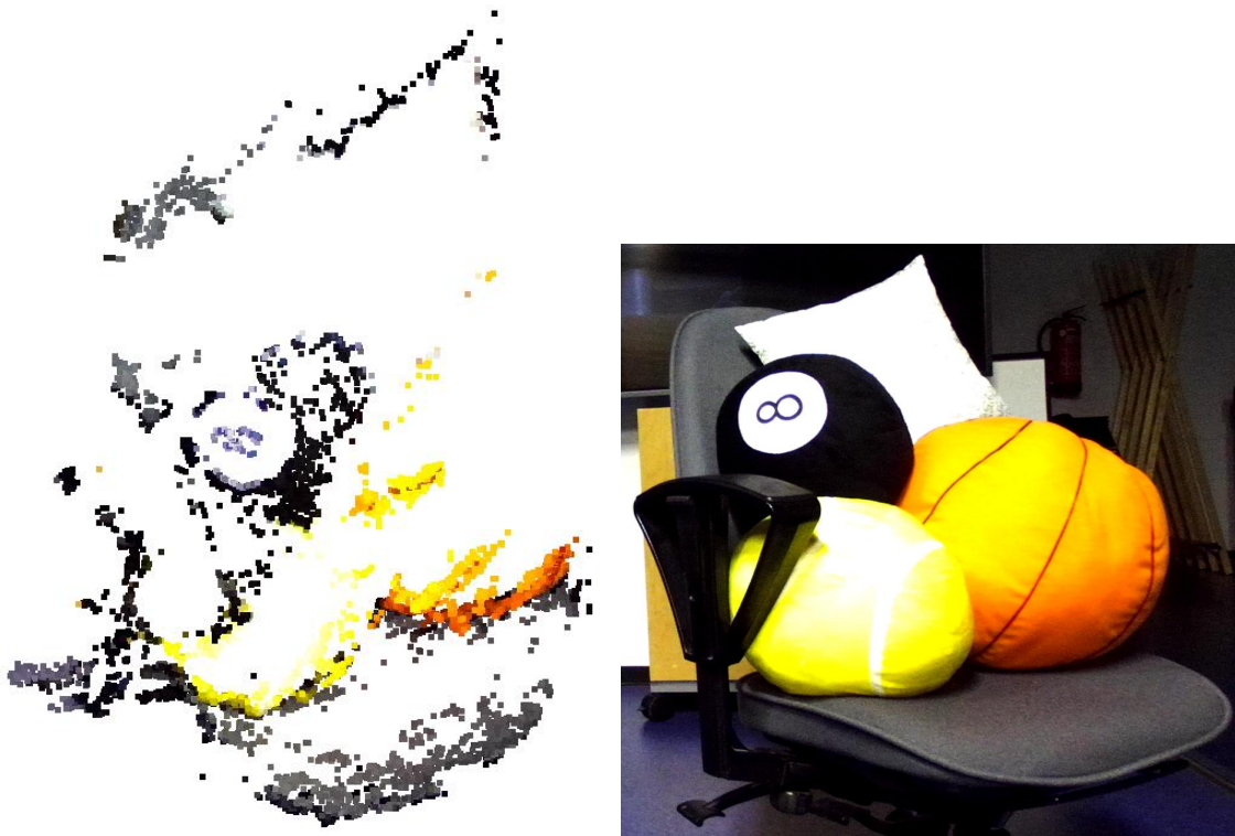
Figure 5.6. Point cloud model produced by our multi-view algorithm and the original object in an image.
