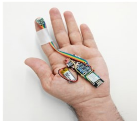
Figure 10. Vital signs measurement with the implemented sensor node
