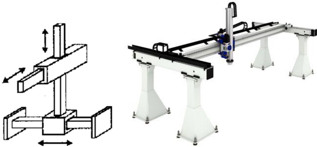
Figure 2. Cartesian robot axis configuration [9] and FlexMotion4 Gantry robot from Automated Motion
