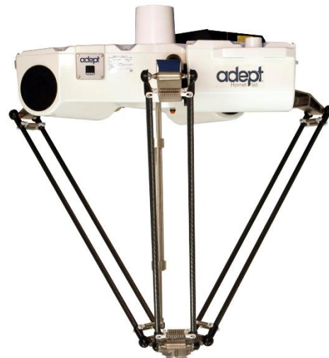
Figure 5. Parallel robot structure [14] and Adept parallel robot from Omron Electronics
