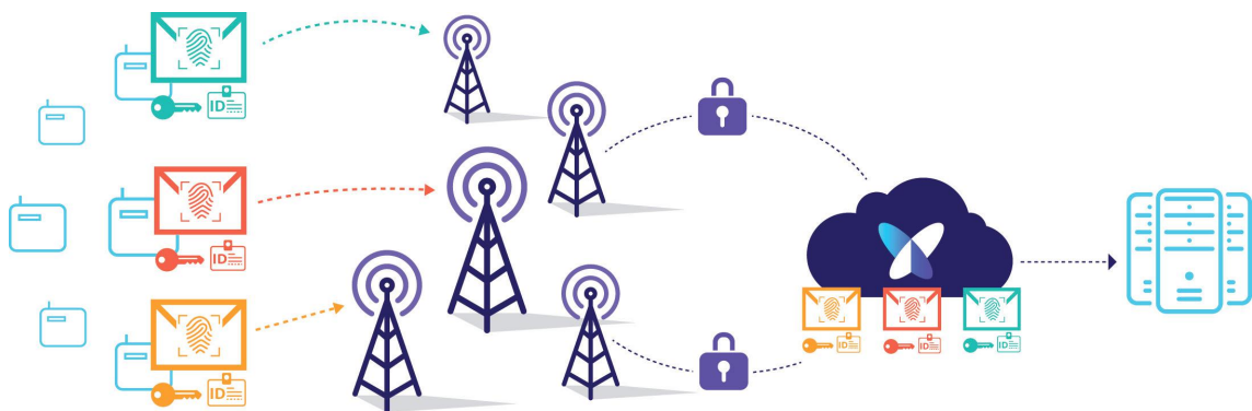
Figure 3.14 Sigfox devices security schematics [5].
