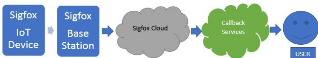
Figure 3.9 Sigfox callback schematics.
