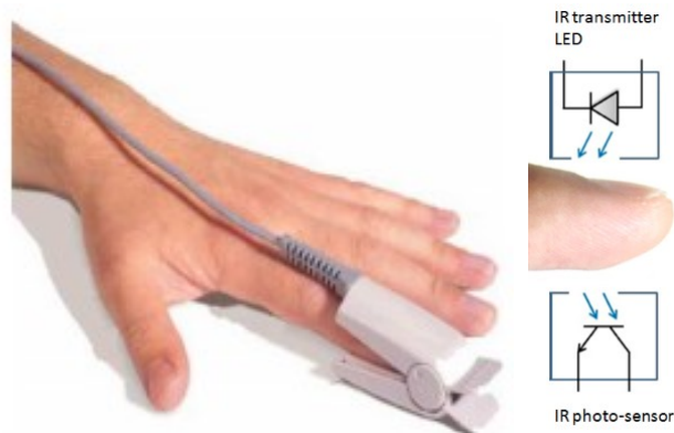
Figure 12. An example of a PPG finger clip sensor, which is using infrared light. Adapted from [58].
