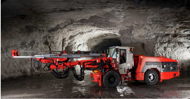
Figure 2: A typical mining rig with a drilling manipulator attached (Photo: Sandvik).
