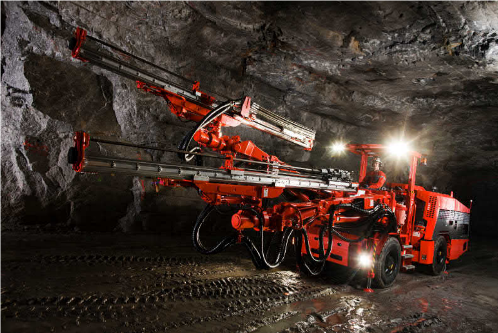
Figure 1.1: Heavy-duty hydraulic manipulators on a drilling rig (Photo: Sandvik) [2].
