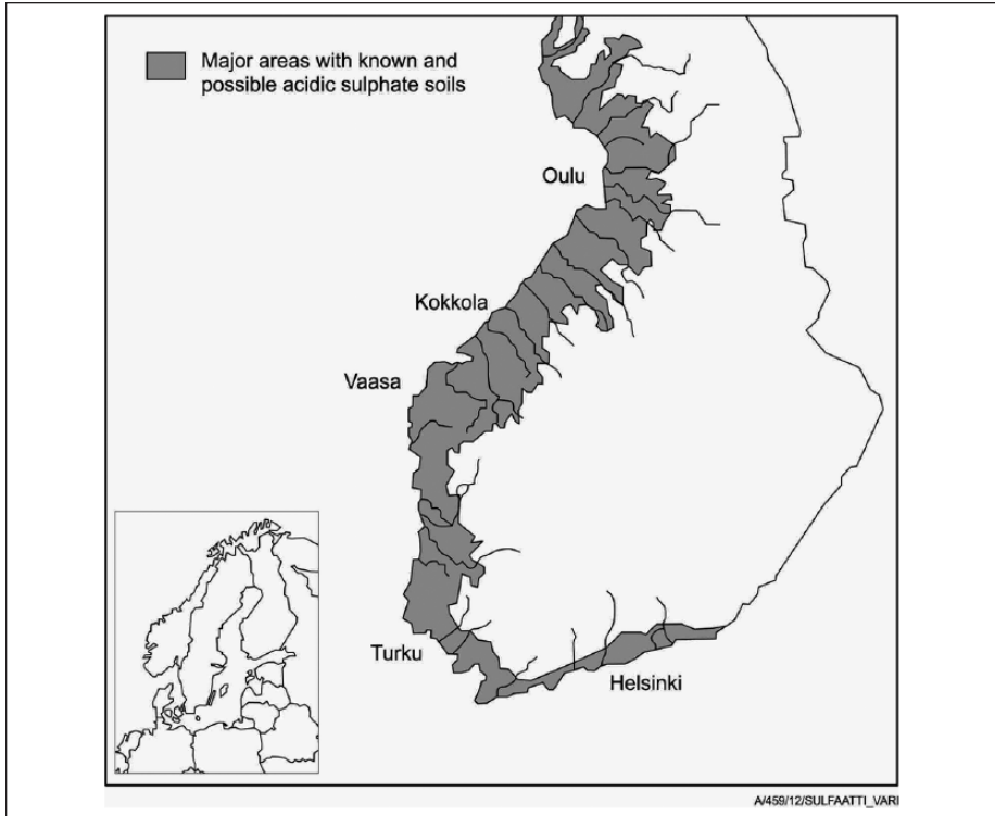
Figure 1. Deposits of acid sulfate soils in Finland, formed during the Litorina stage of the Baltic Sea about 7500-1500 BC.
