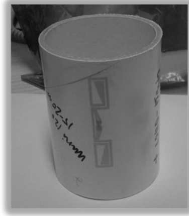
Fig. 6.2. Prototype tag printed directly on cardboard reel with pad printing.
