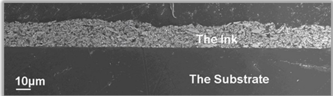
Figure 4.5. SEM micrograph of Sample 2 in article [P5], average thickness 21.5 \mu\text{m} .
