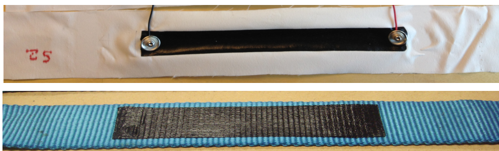
Figure 8. Examples of conductive rubber coated samples on elastic woven fabrics (top) and inelastic cargo strap (bottom).
