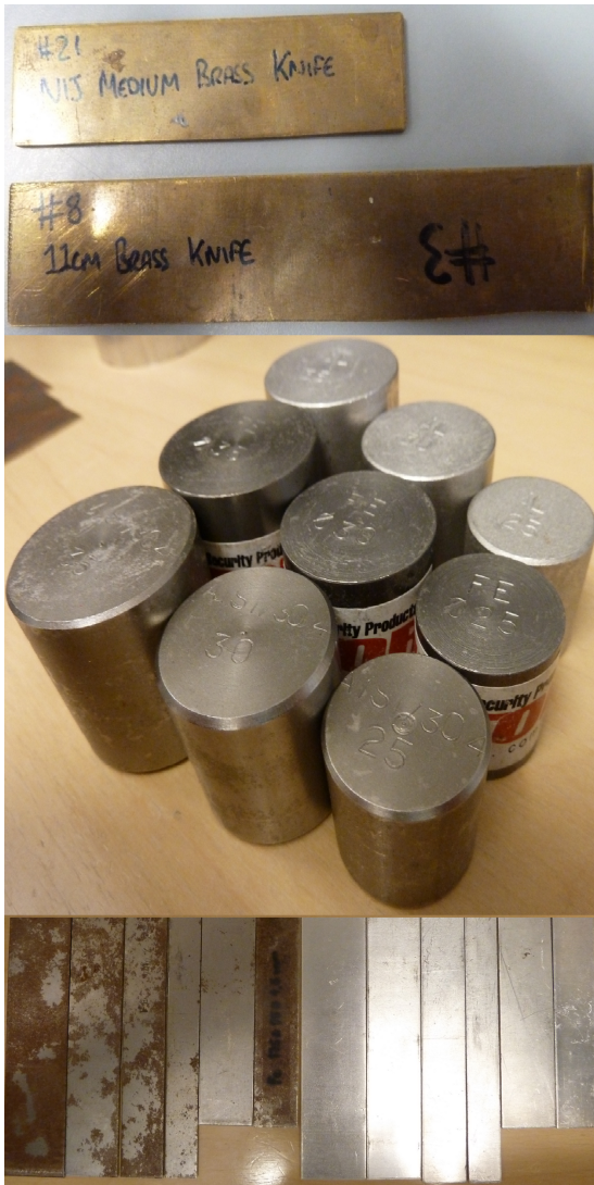
Fig. 3. Brass strips, aluminium, iron, and stainless steel cylinders, and iron and aluminium strips.
