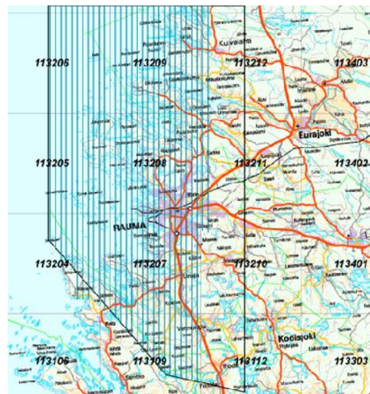
Figure 2. A map demonstrating the flight lines over the test area.
