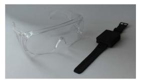
Figure 1. Device surrogates used in the study: smartglasses (left) and smartwatch (right).
