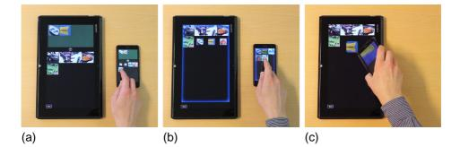
Figure 4.5: Different cross-display object movement methods: (a) Tray: a user moves objects by dragging them to and from a virtual tray shared between all devices. (b) Transfer Mode: a user first sets up a connection between devices by making a screen gesture and then shares objects between devices by simply tapping objects on the displays. (c) Device Touch: a user moves objects by physically touching the screen of another device with the corner of the phone.
