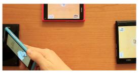
Figure 3. The Host method. The user holding the cyan device has connected the black (right) and magenta devices (top).
