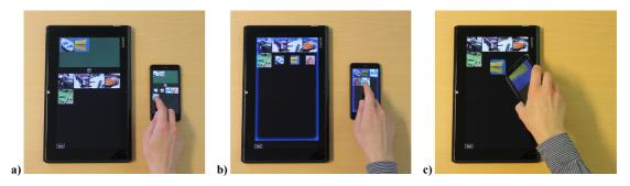
Figure 1. Different cross-display object movement methods: a) Tray, b) Transfer Mode, and c) Device Touch.
