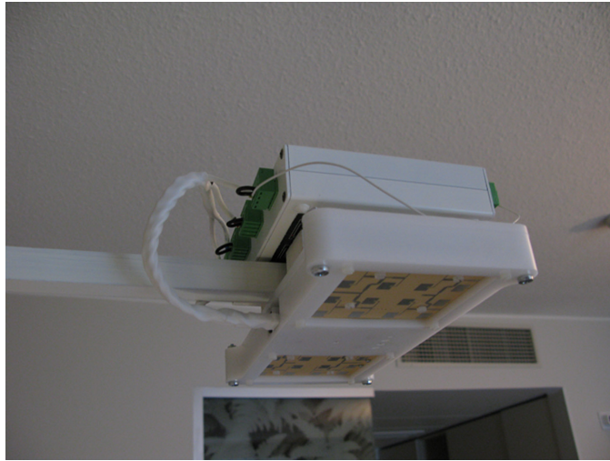
Figure 3.3: The radar sensor attached in a stand. The two radar modules are attached side by side, the amplification circuit is in the middle of the radars, and the ADC card is above.
