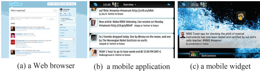
Figure 1.1. Three conventional UIs for accessing Twitter on the Nokia N900 device: a mobile Web browser (a), a dedicated Twitter application (b), and a mobile widget (c).
