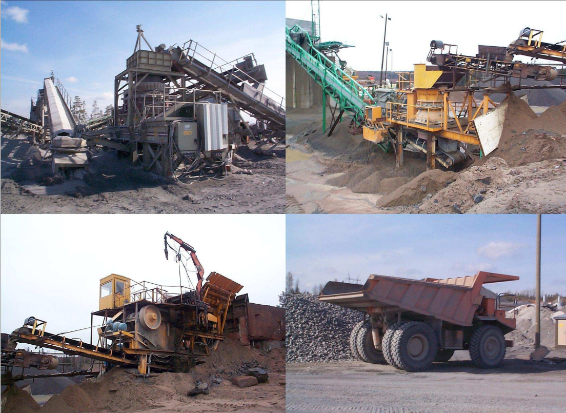
Fig. 1.2: A rock-crushing station has many distinct noise sources, among them cone and jaw crushers, stone screening and conveyor systems, excavators, front-loading shovels, dozers, and haulage vehicles [75] . Image © 2003 V. Mellin; used with permission.
