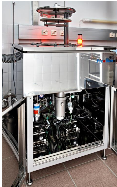
Figure 6. An example of atomic-layer-deposition (ALD) device.
