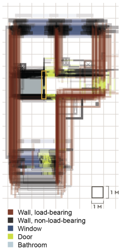
Figure 3. A pile of colour-coded graphs for flat type 2-1A. Line weights and colours distinguish different elements of the plan. In the image, the graphs have been aligned along the circled bathroom wall. The colour key also applies to Figures 4–8.
