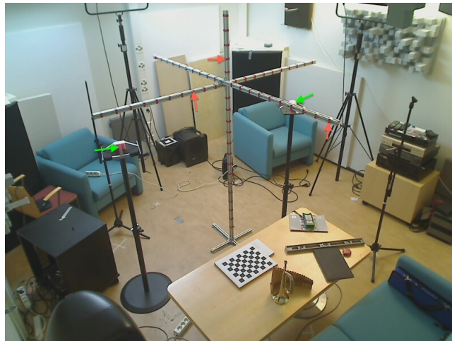
Figure 3.5. The frame with calibration marks. The calibration points are highlighted by the red arrows and are visible to four cameras that used to obtain the reference 3D coordinates (see [P1] for details). The two points highlighted by two green arrows outside the calibration pole are also used to increase the accuracy of the transformation.
