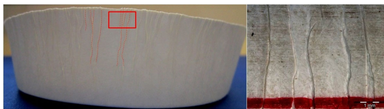
Figure 4. The formed shape with wrinkles and microscope image of the wrinkles.
