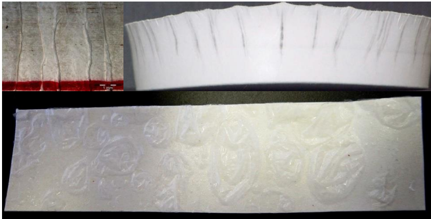
Figure 9. Upper image: discoloration in deep-drawn shapes (left), discoloration coupled with earing (right), courtesy of M. Hauptmann, Lower image: blistering of the fragment of the tray trim in thermoforming process.
