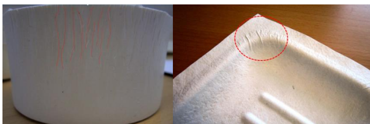
Figure 8. The wrinkling in the side wall of a deep-drawn shape (sliding blank) (left) and flange wrinkling in a shape produced by hot pressing (fixed blank).
