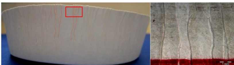
Figure 15. Photographical images of the formed shape with wrinkles and a closer magnification image of the compression wrinkles.
