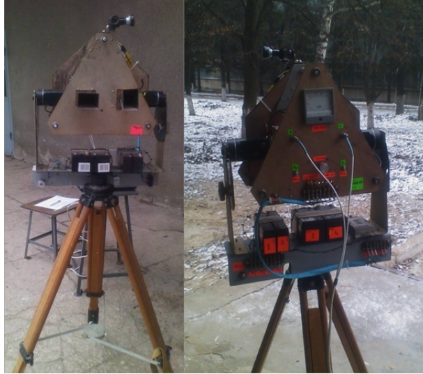
Figure 5.17: Ground surveillance radar system used for experimental data collection.
