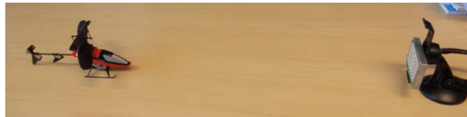
Figure 3.6: Experimental setup of micro-Doppler signal collecting from rotating blades of a toy helicopter.
