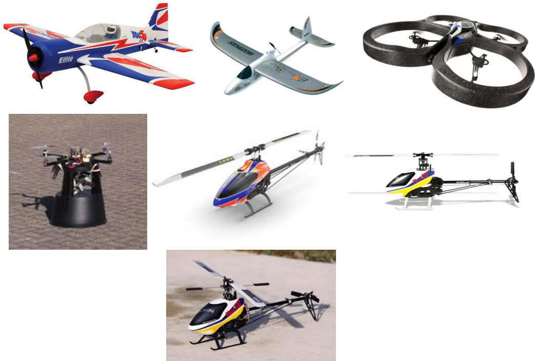
Figure 7.6: Examples of UAVs used for experimental study, from left to right, from top to bottom: YAK54 (class 1), EasyStar El-Sailor (class 2), Parrot AR.Drone (class 4), stationary rotors (classes 5-8), Mikado Logo 600 (class 9), Mikado Logo 400 (class 10), Align T-REX 450 (class 11).
