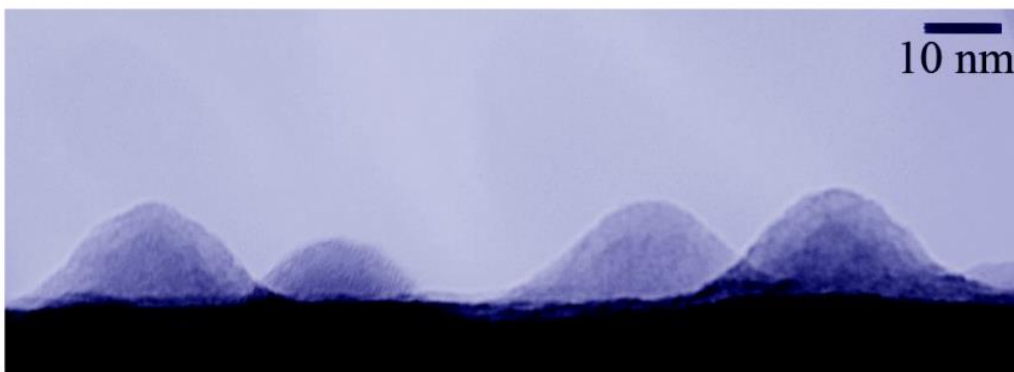
Figure 1.3 Cross sectional transmission electron microscope image of InAs quantum dots on GaAs [17].
