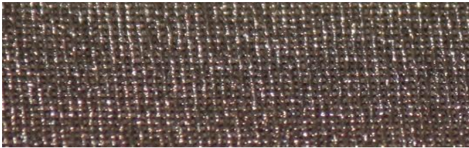
Figure 22. Material 2 C: Silver coating on a knitted structure.
