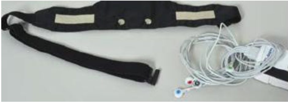
Figure 14. ECG belt with a continuous electrode-moisturizing element. [66]
