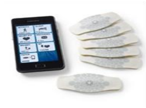
Figure 9. Detachable, disposable electrodes are one competing technology for textile electrodes. The application uses a smartphone as a user interface. [100]
