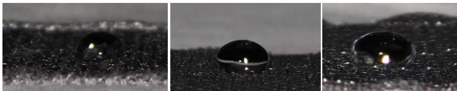
Figure 56. Specimen 3 C with untreated, Nano-X treated and unwashed, and 20 x washed surfaces.
