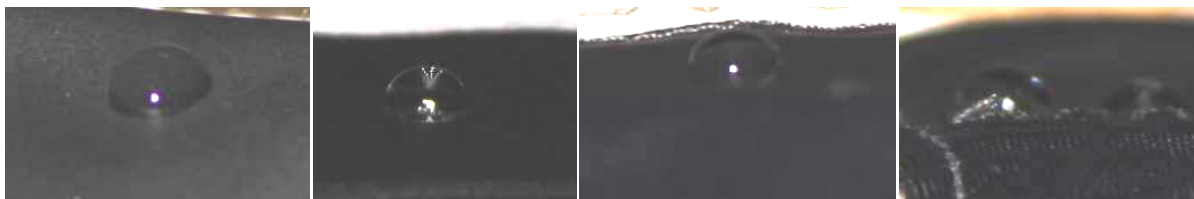
Figure 60. Specimen 6 NK with untreated, Nanotex-treated, 20 x washed, and 20 x sterilized surfaces.
