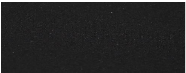
Figure 26. Material 6 NK: TPU-coated interlock knit.
