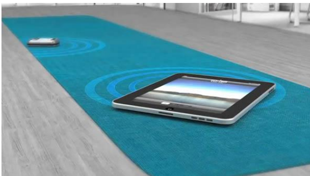
Figure 8. The Powertex textile is an inductive recharger for mobile devices. [34]
