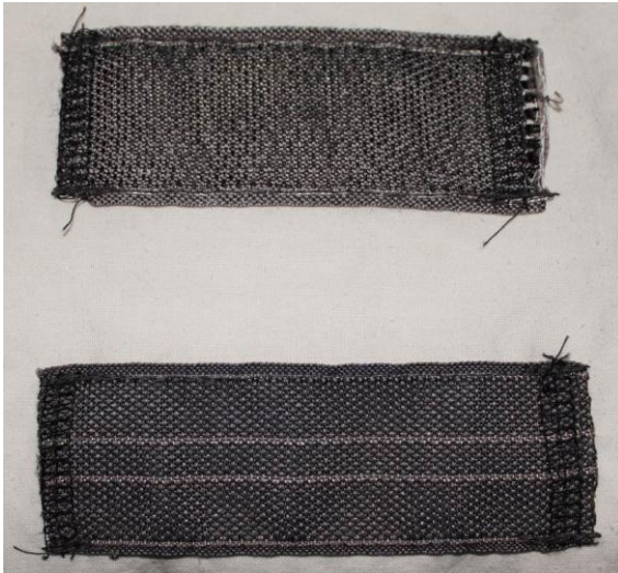
Figure 37. Materials 4 C (above) and 3 C (below) machine-washed 20 times at 40°C.
