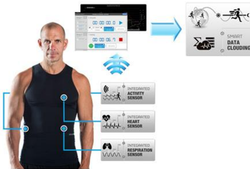
Figure 4: Hexoskin textile heart rate-monitoring operation system. [48]
