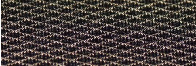
Figure 21. Material 1 C: Silver-plated PA fibre in a warp knitted structure.
