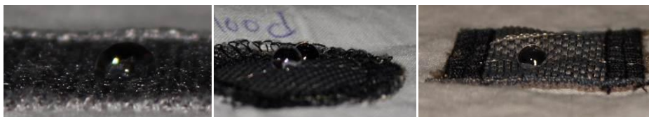
Figure 57. Specimen 3 C with untreated, Nanotex 20 x washed, and 20 x sterilized surfaces.
