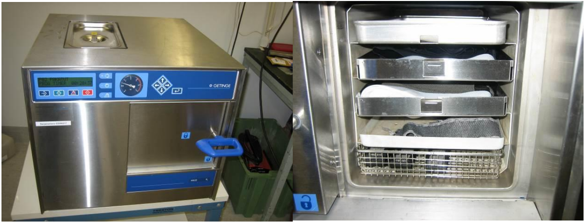
Figure 31. On the left, the autoclaving device used for textile sterilization from the outside. On the right, the textile products to be sterilized are in the autoclave chamber.
