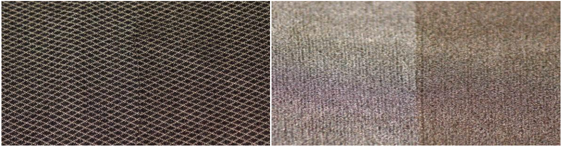
Figure 47. Slight brownish effect after Nanotex treatment for materials 1 C (left) and 2 C (right).
