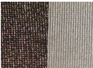
Figure 34. The conductive-coated specimen 2 C before hot steam sterilization treatment on the left, and the delaminated specimen after 5 cycles of sterilization on the right.
