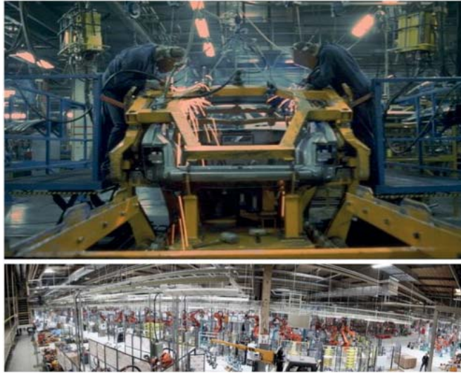
Figure 44. In the upper picture welding of Saab 9000 CC (Combi Coupe) in 1980's and beneath almost finished preparations for a new car model production in 2010's.
