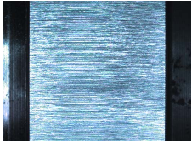
Figure 12. The test disc surface has been finished perpendicular to the rotating direction.
