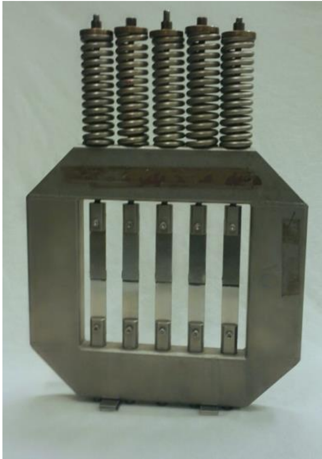
Figure 24. Test rig used for the static loading of the single lap joint specimens during the aging exposure.
