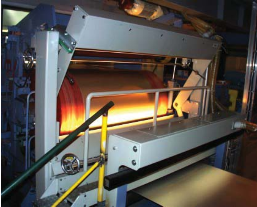
Figure 2.3. A surface inspection system monitoring metal strip quality.
