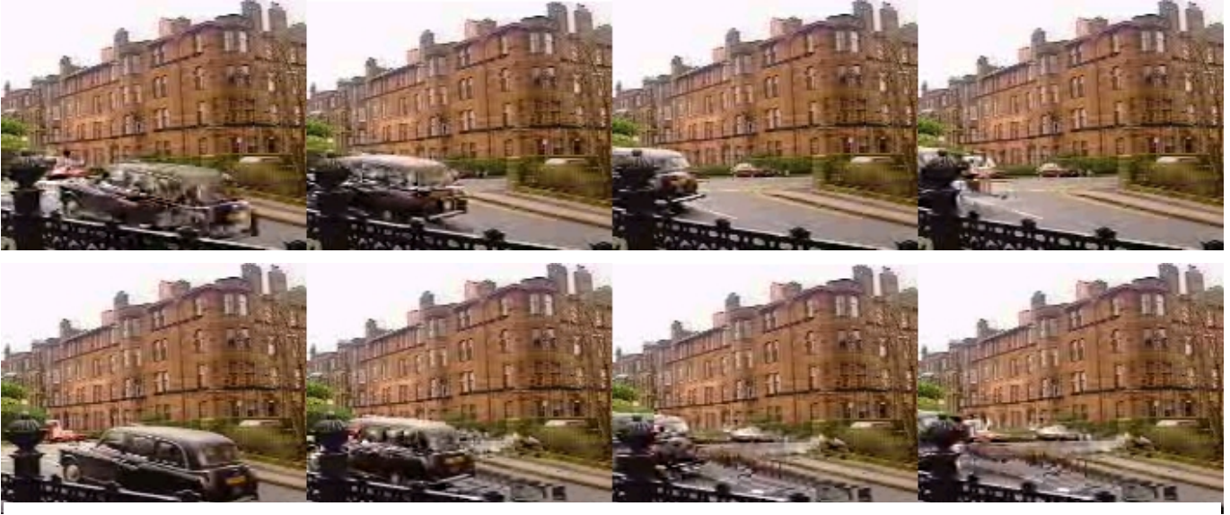
Figure 5. Reconstructed frames of an example scene. The top row shows frames reconstructed from a sequence coded according to the INTRA frame postponement method. The bottom row is conventionally coded.
