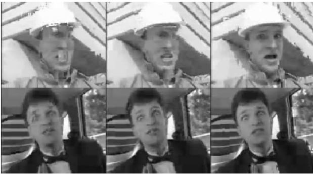
Fig. 7. Results of the unequal error protection simulations: example snapshots of 20% packet loss rate. From left to right, the used codecs are Conv, Conv + ROI, and the proposed codec.
