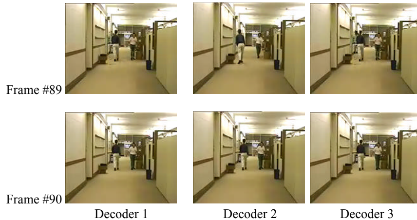
Figure 5. Snapshots of Hall @ packet loss rate 5%, 16 frames before frame 90 are frozen by Decoder 2 and rescued by Decoder 3
