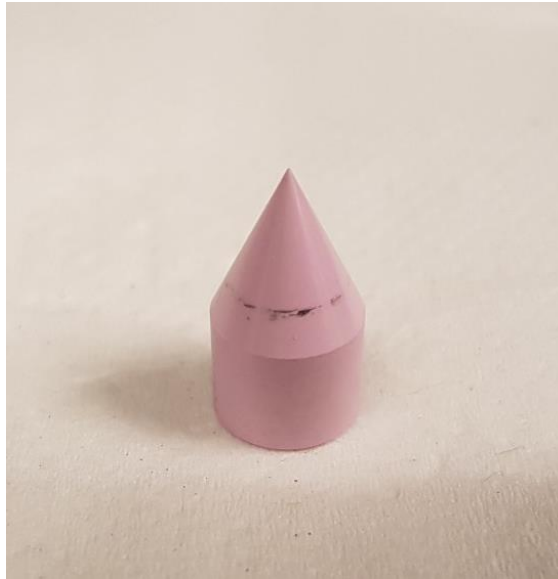
Figure 12: Typical nozzle of Nscript 3D dispensing system.
