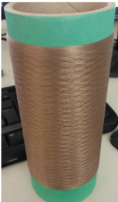
Figure 2. Melt spun SPEEK/PP 5 : 95 filaments. [Color figure can be viewed in the online issue, which is available at wileyonlinelibrary.com .]
