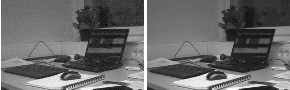
Figure 5.2: Denoising of a raw image acquired with a Nokia N9 smartphone at ISO 3200. Left: noisy image. Right: denoised image.
