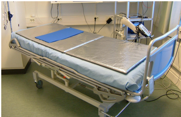
Figure 1. The blue Emfit- mattress on top of the traditional SCSB-mattress (coated silver foil). In clinical use, they both are placed under a normal foam mattress.
