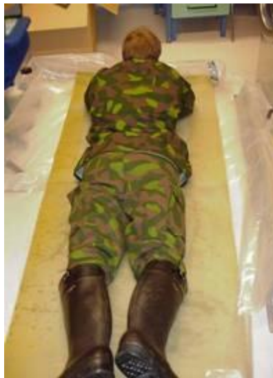
Figure 1. The test subject lying on the water absorbed mattress during the moisture retention tests.
