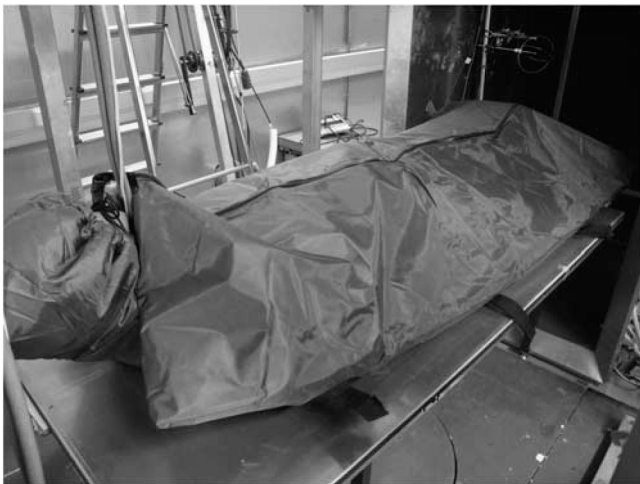
Figure 1. Measuring Thermal Insulation of Protective Coverings Using Supine Thermal Manikin on Metal Sheet
