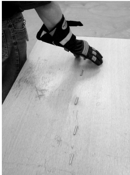
Figure 5. Finger dexterity tests with different gloves using five test pins
