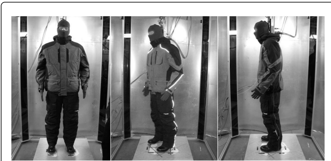
Figure 2: Effects of wind direction (wind speed 8 m/s) on effective thermal insulation ( I_{cle} ) of clothing ensemble C3, tested at angles of 0°, 45° and 90° to the wind.
